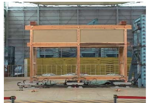
When the circumference of the post is a size thinner, the post snaps. If the plinth slides, however, there is little damage.
