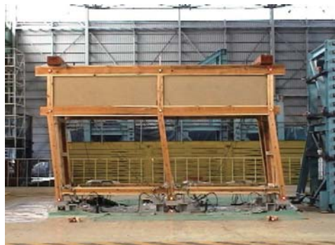
When the circumference of the post is a size thinner, the post snaps. If the plinth slides, however, there is little damage.
