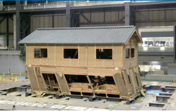
Vibration testing of a two-story full-size wooden home. (Research project by the Ministry of Land, Infrastructure, Transport and Tourism, 2008.)
