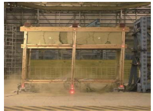
Test situation: When the logs are thick, the wall in the upper section is destroyed.
