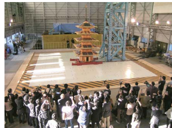
Vibration testing of a mockup of a five-story pagoda. (Forum for Wood Architecture and the National Research Institute for Earth Science and Disaster Prevention, 2004.)
