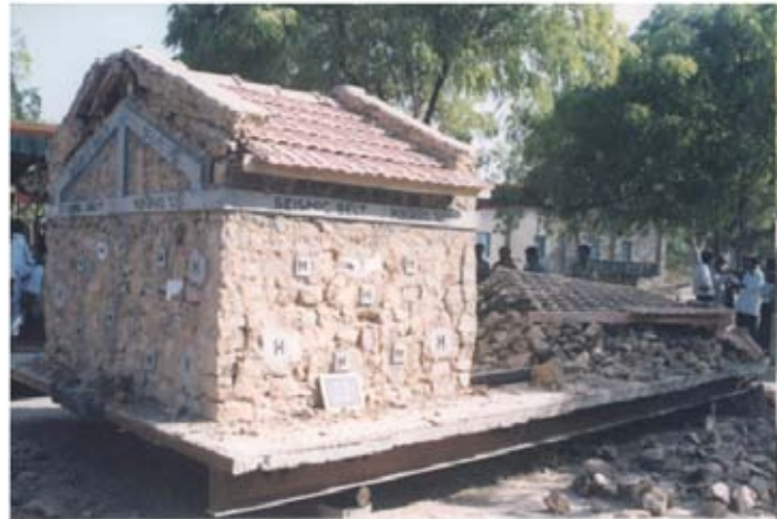
Shock No: 11, T.M Collapse, I.M End Wall Cracked
