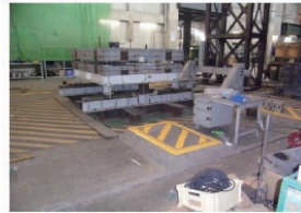
Shaking Table in BRI used for the experiments
